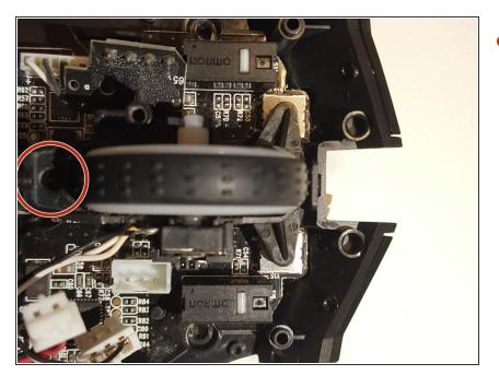
Using a Phillips #00 screwdriver, remove the single screw adjacent to the wheel.
