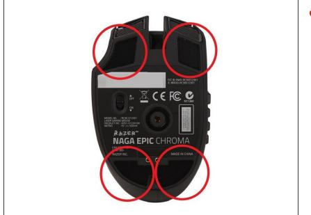
Using a spudger, remove the teflon tape on the bottom of the mouse to reveal four screws.
