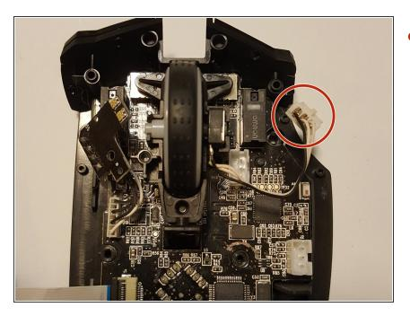
Unplug the wheel cable connecting to the board.
