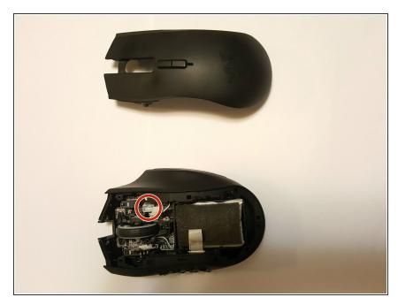
Plug the new top casing's cable back into the socket on the right side of the circuit board near the middle.
