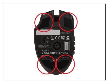
Using a spudger, remove the teflon tape on the bottom of the mouse to reveal four screws.
