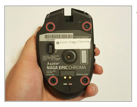
Use a Phillips #00 screwdriver to remove the four screws.
