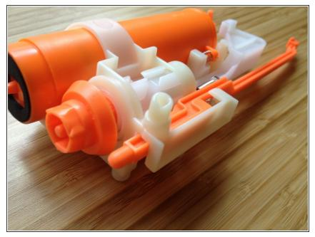
The rough white cylinder circled in red on this picture will be covered in some grease. Do NOT wash it off.
