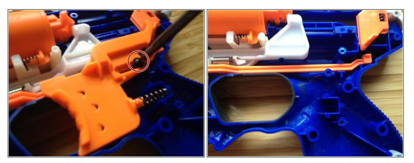
(i) Remove the screw that holds the trigger in place.
