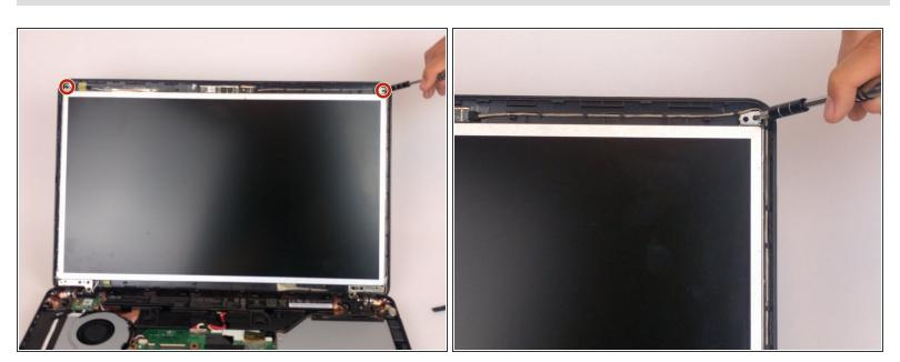
• Remove the two 4.7mm Phillips#00 screws to free the screen-holding bracket from the back panel.
