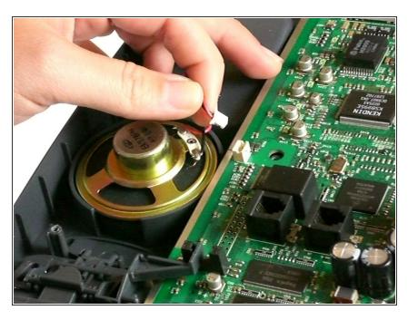
While holding down the motherboard, gently pull the wire harness connecting the speaker to the motherboard until it comes free.
