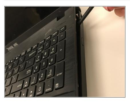
Pry up the keyboard using a plastic spudger.
