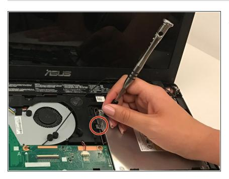
Remove the four, 4 mm screws using a Phillips #00 screwdriver.
