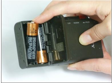
Lift the cover and remove the batteries.
