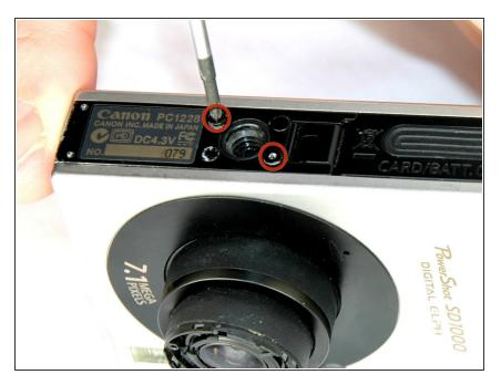
Remove the two 2.9 mm screws from the camera bottom panel.
