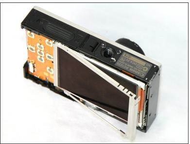
Pull up the metal frame surrounding the LCD screen starting at the side of the camera.
