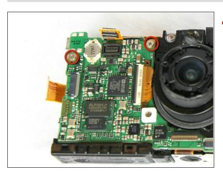
Remove the two 2.90 mm screws from the motherboard.
