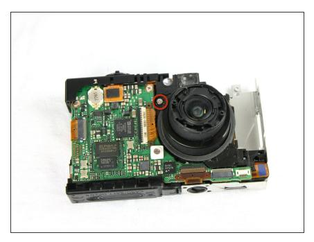
Remove the 2.90mm screw from the lens, near the motherboard.
