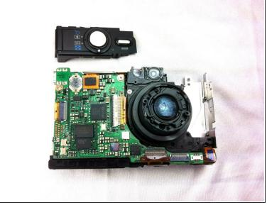
Using the spudger remove the shutter button by prying the small tab on the front side of the camera.
