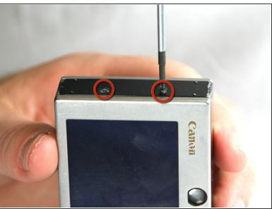
Remove the two 2.9 mm screws from the side panel closest to the camera lens.
