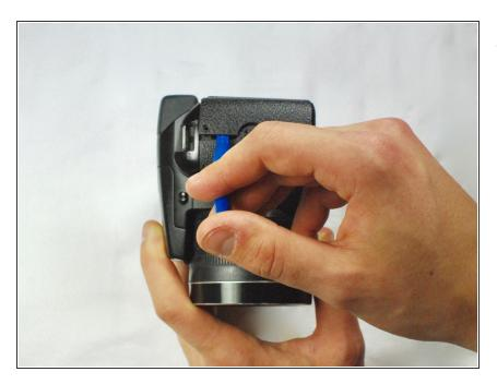
• Use a plastic opening tool to separate the back panel from the camera on the left side.
