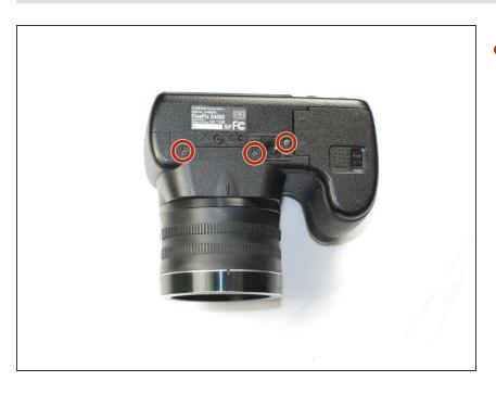
Remove the three 3.5 mm Phillips #1 screws in these locations on the bottom of the camera with a screwdriver.
