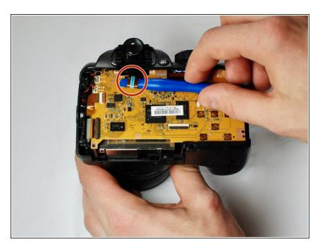
Use the plastic opening tool to remove the ribbon wire from inside the camera
