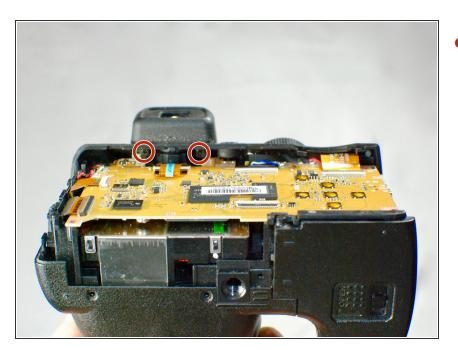
Turn the camera on its side and remove the highlighted 2.7 mm Phillips #1 screws.
