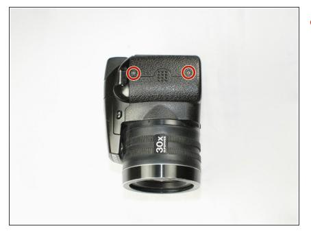
Remove the two 3.5 mm Phillips #1 screws in these positions on the left side of the camera with a screwdriver.
