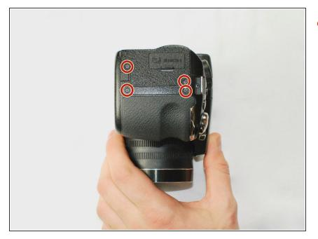
Remove the four 3.5 mm Phillips #1 screws in these positions on the right side of the camera with a screwdriver.
