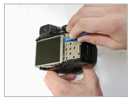
Use a plastic opening tool to separate the LCD screen from the camera.
