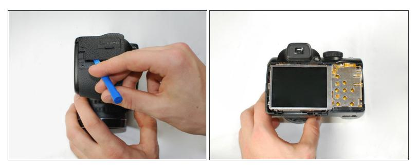
• Use a plastic opening tool to separate the back panel from the camera on the left side, then remove the back panel from the camera.
