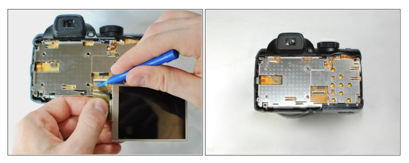
• Flip up the black tab holding the LCD ribbon wire in place and remove wire.
