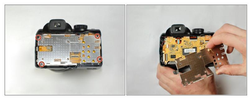
• Remove the highlighted 2.7 mm Phillips #1 screws to release the metal cover.
