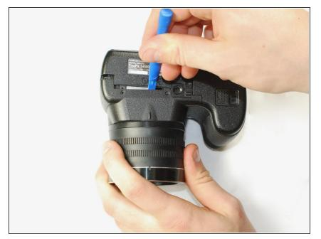
• Use a plastic opening tool to separate the back panel from the camera on the bottom.
