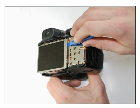
Use a plastic opening tool to separate the LCD screen from the camera.
