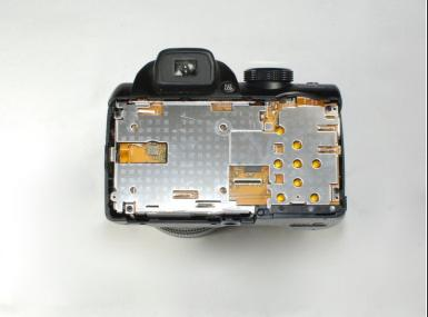
• Flip up the black tab holding the LCD ribbon wire in place and remove wire.
