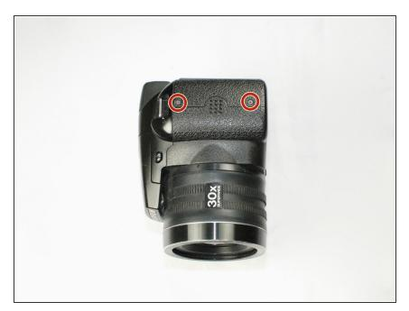
Remove the two 3.5 mm Phillips #1 screws in these positions on the left side of the camera with a screwdriver.
