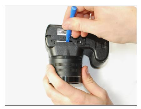
Use a plastic opening tool to separate the back panel from the camera on the bottom.
