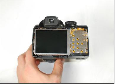
Use a plastic opening tool to separate the back panel from the camera on the left side, then remove the back panel from the camera.
