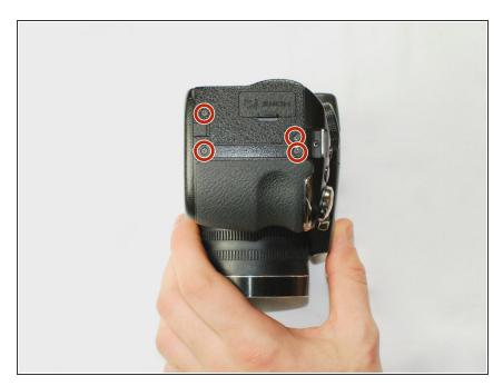
Remove the four 3.5 mm Phillips #1 screws in these positions on the right side of the camera with a screwdriver.
