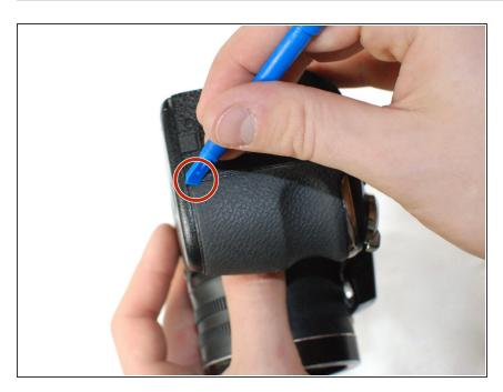
Use a plastic opening tool to pry up the corner of the grip.
