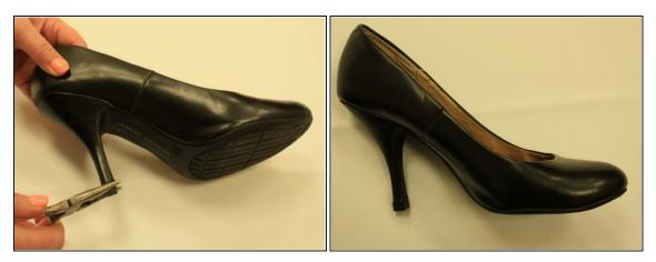
• Adjust the tip with the pliers to align the heel tip.
