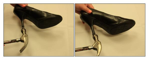
• Gently tap the new tip in with the hammer. Careful not to damage the shoes material.
