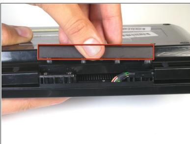
Use your hand to remove the small back cover by gently pulling upward.
