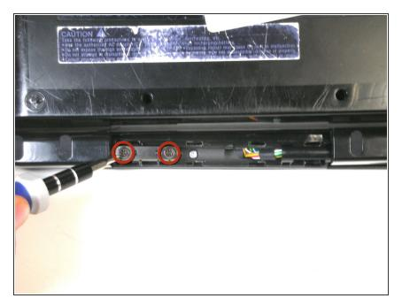
Using a screwdriver, remove the two
