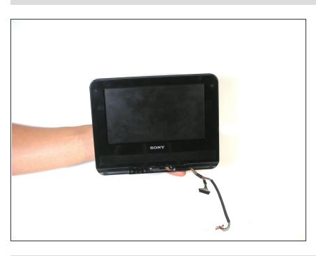
The screen should now be completely separated from the main device.
