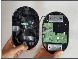
Remove the screws (11.27mm Phillips head) and open up the transmitter to reveal the internal components. Carefully pry open the transmitter, and use caution when opening it up as to not sever the wire.
