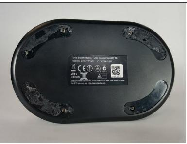
Begin by flipping over the transmitter, and removing the padding from the underside of it. This will
