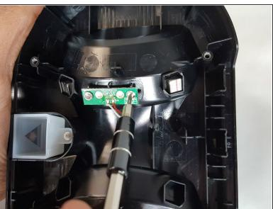
Remove the two screws (5.21mm Phillips head) on the board on the top half of the transmitter that is holding the charging pins.
