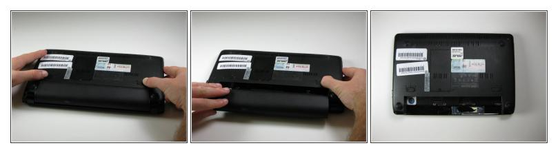
• Slide the tabs outward to unlock the battery.
