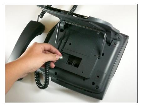
Before disassembling the phone, make sure it is not plugged into power and the handset phone cord is disconnected from the handset jack.
