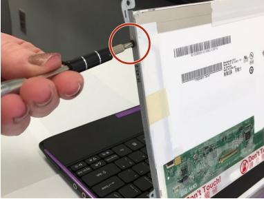
Remove the two 6mm screws on each side of the screen with a Phillips #0 screwdriver.
