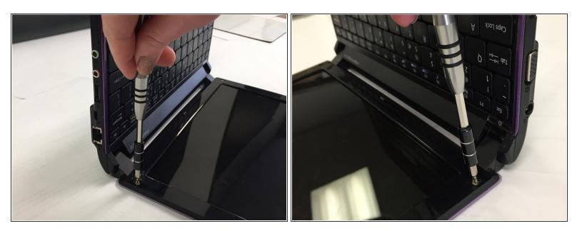
Use a Phillips #0 Screwdriver to remove the two 6mm screws from the screen.
