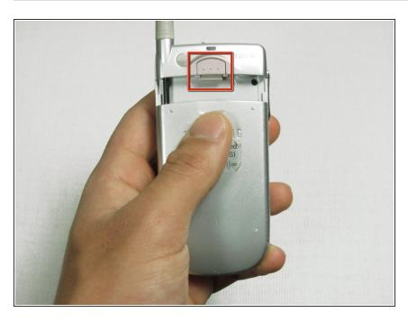
Remove the battery by pressing the button at the top of the case.
