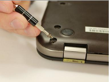
Using the #PH0 screw head, remove 14 (5.7 mm) screws from the back casing.
