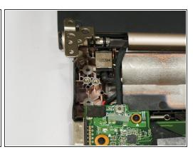
Remove one (1) 5mm x 4mm screw from the upper left hand corner of the motherboard with the size 0 Phillips screwdriver.
