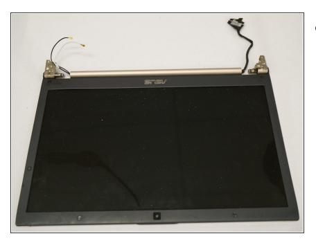
Lift up the corner of the motherboard on both sides and disconnect the wires connecting the screen by pulling gently.
