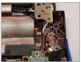
• Remove two (2) 5mm x 4mm screws from the upper right hand corner of the motherboard with the size 0 Phillips screwdriver.
