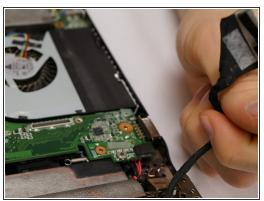
• Use the straight tweezers to disconnect the wires attaching the screen to the main computer by pulling up gently. The computer screen should be open and away from you.
