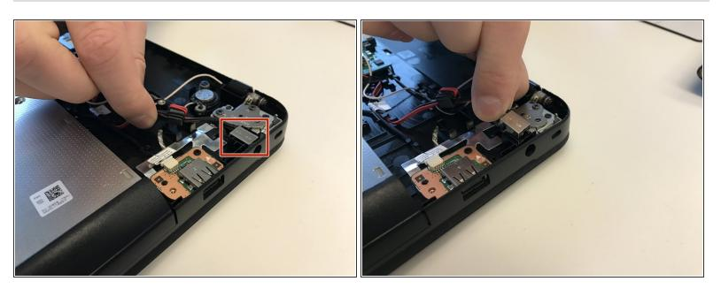
Remove the DC power jack from its plastic retaining piece, just inside of the charger inlet.
