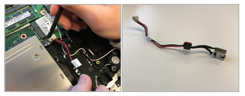
Use the nylon spudger to remove the connecting wires from the motherboard. Insert the spudger between the terminal plastic piece of the wire and its retaining clip on the mother board. The wire should release without much force. To reassemble your device, follow these instructions in reverse order.
