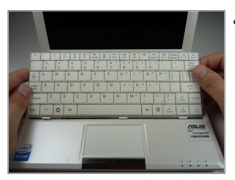
Remove the keyboard by lifting upwards.
