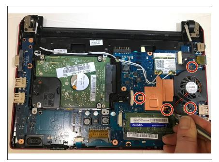
Remove the four 6.5 mm screws that surround the fan using the PH1 Phillips screwdriver head.
