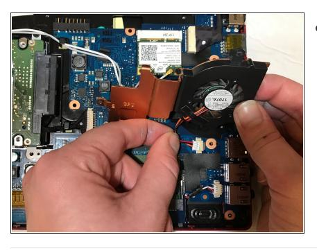
Manually remove the fan from the device by pulling out the connector.
