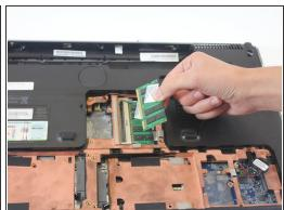
• Remove the green RAM by prying it upward and pulling it away from its slot.
