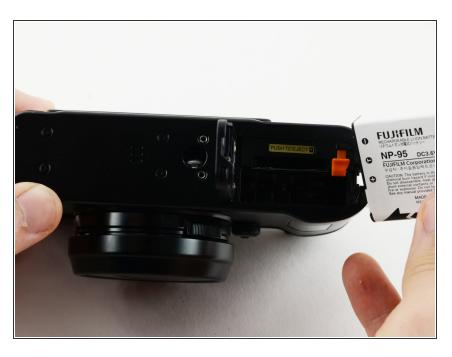
First line of business: Remove power from the camera. Remove the battery from the X100t.
