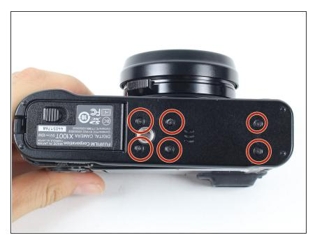
Unscrew the six 4.0 mm JIS#00 screws on the bottom of the camera.
