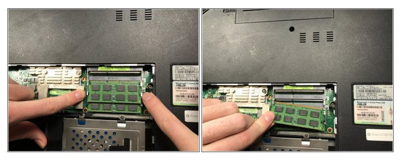
Push down the metal clips and remove the RAM.
