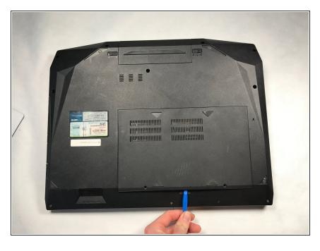
Use the plastic spudger to remove the panel.
