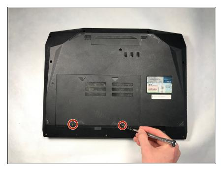
Locate the two, 4mm screws on the back of the laptop and remove them using a PH0 screwdriver.
