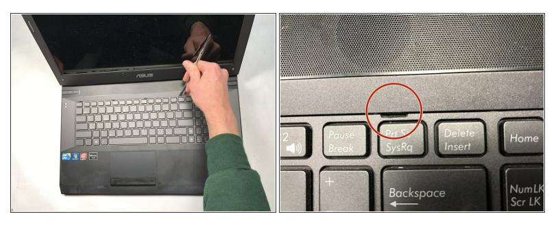
Locate the 5 clips located at the top of the keyboard. Insert a metal spudger into the clip openings on the keyboard to remove the keyboard.
