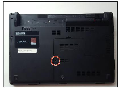
Locate and remove the 8mm PH0 screw near the middle of the laptop.
