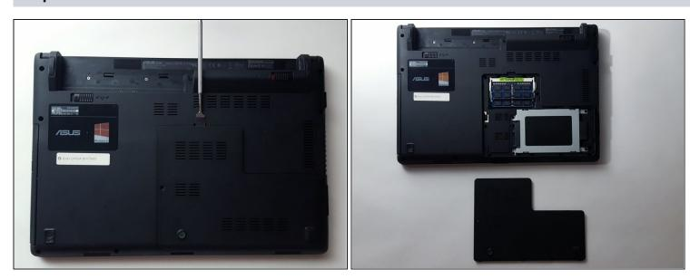
• Use a metal opening tool to remove the L-shaped, plastic cover.
