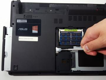
On the left side of the section, there is a metal tab. Using a metal opening tool, push the tab as far as possible to the left.
