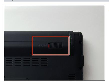
In the top right corner, push the tab to the right to the unlocked position.
