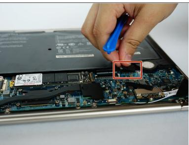
Disconnect the battery from the motherboard by gently pulling up and down on the connector.
