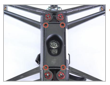
Remove the four 5mm torx T5 screws on the bottom of the drone with a Torx Screwdriver.
