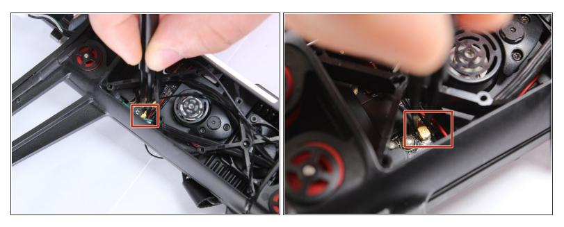
Using a small pair of tweezers remove the two antenna wires attached to the motherboard.
