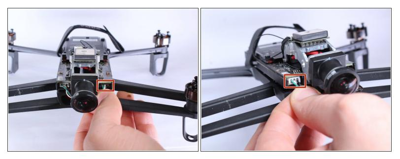
Disconnect the two connectors that are attached to the front of the motherboard by gently pulling on the three wires.
