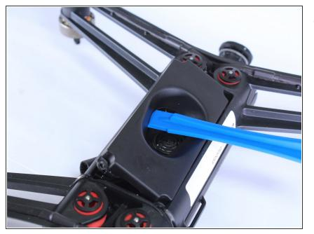
Lightly pull up using the plastic opening tool to remove the back cover.
