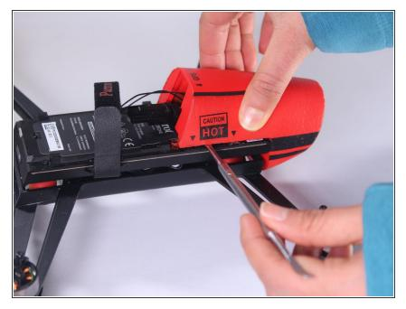
• Take the metal spudger, to remove the double stick tape from the foam.
