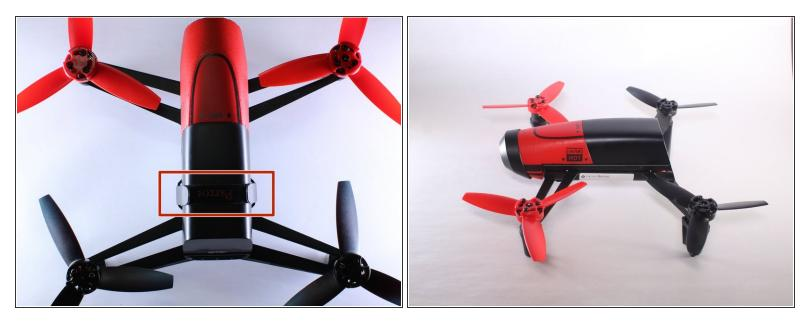
• Begin by removing the velcro strap around the battery.
