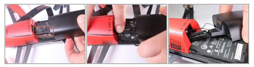
Once the battery is separated from the nose, push down on the connector and pull the battery away from the connector.
