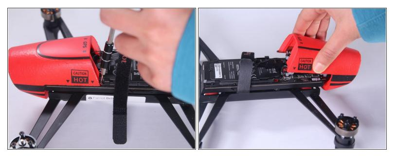
• Remove the two 7mm T5 torx screws using a screwdriver. There is one located on each side.
