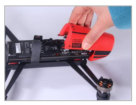
Remove the styrofoam nose from over the drone's camera by sliding it towards the front of the drone at an angle.
