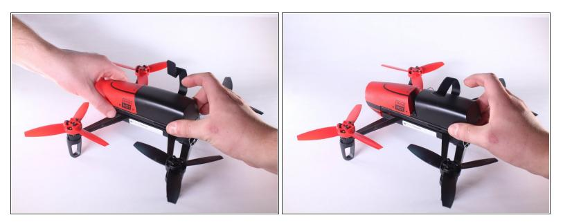
• While holding onto the nose, gently pull the battery away from the nose.
