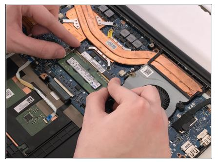
• Place fingers on metal clamps that hold the RAM stick in place.
