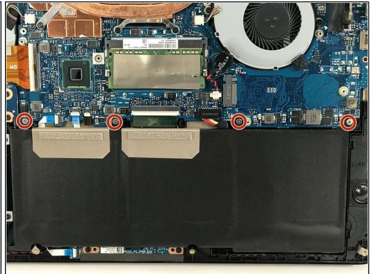
⚠️ Attach the clip of your [anti-static wrist strap](#) to the case of the laptop. This prevents any accidents that could fry the motherboard.
