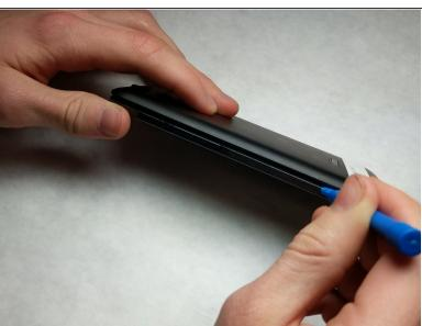
Pry off the back cover with the blue plastic opening tool. This may require a bit of force.
