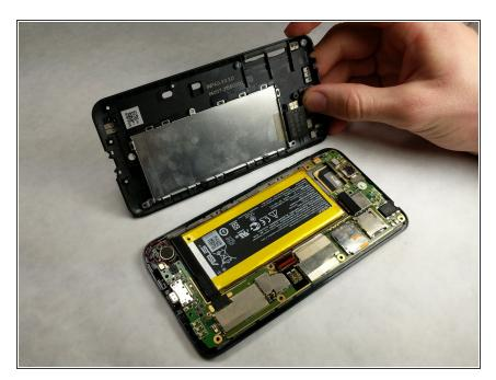
Once the screws are removed, the mid-frame can be lifted off of the phone. The speaker is on the midframe.
