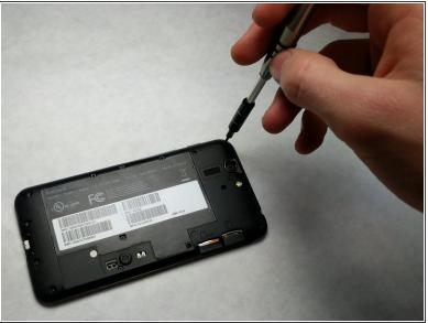
Remove the thirteen 3.6mm screws using the T5 Torx Screwdriver.
