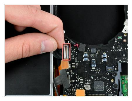
• Disconnect the display data cable by pulling the male end straight away from its socket.
