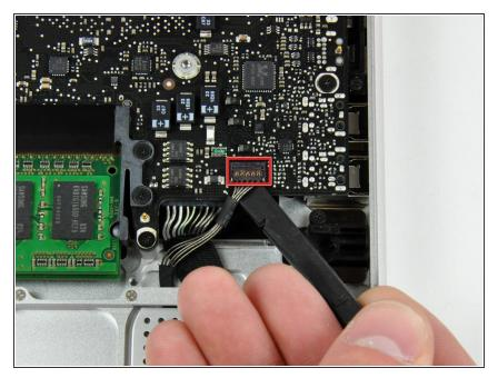
• Use a spudger to pry the battery level indicator cable connector straight up off the logic board.
