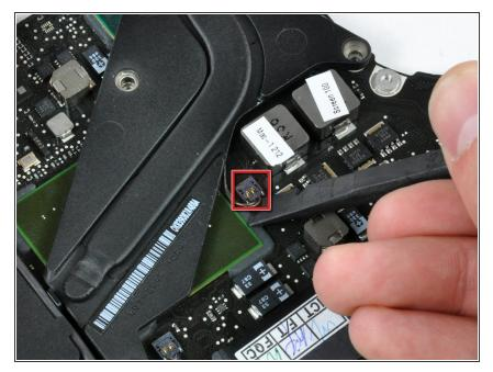
• Use the flat end of a spudger to pry the thermal sensor connector up off the logic board.
