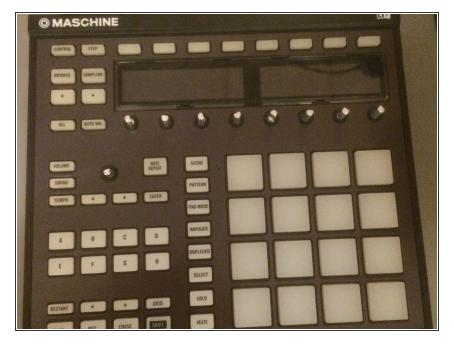
since we don't know if we're going to remove the PCB, or if it's fixed to the knobs, it's best to remove all plastic caps
