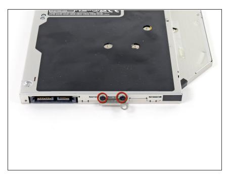
Remove the two black Phillips #0 screws securing the small metal mounting bracket. Transfer this bracket to your new optical drive or hard drive enclosure.
