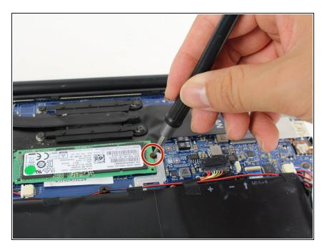
Remove the black, 4 mm Phillips screw securing the SSD.
