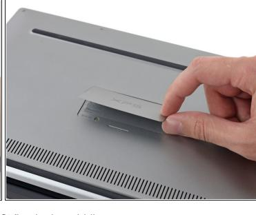
• Use a plastic opening tool to pry open the 'XPS' flap in the middle.
