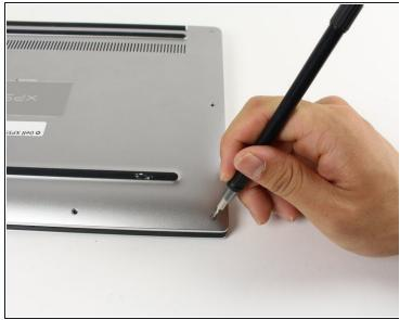
Remove the eight 4 mm T5 Torx screws from the bottom cover.
