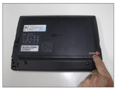
Unlock the battery by sliding the indicated lock to the right. A red indication will show it is unlocked.
