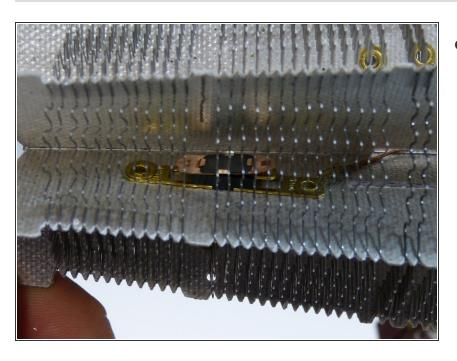
Replace the old thermal fuse by a new one.
