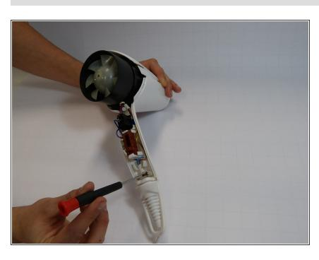
Unscrew the remaining two screws inside the handle with the Phillips screwdriver.
