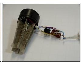
Push the inner components out of the handle.
