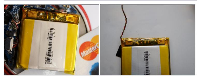
• You can take the battery out by using a <u>plastic card</u> such as a credit card
