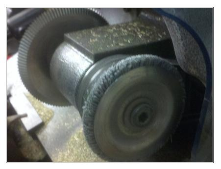
As you can see, the deburring wheel on this machine is quite worn down. Time to replace!
