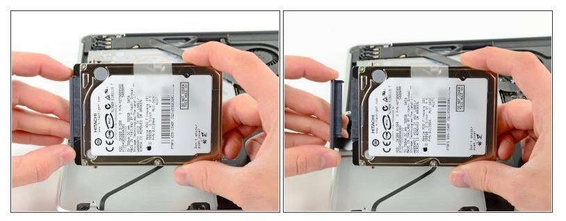
• Remove the hard drive cable by pulling its connector straight away from the hard drive.
