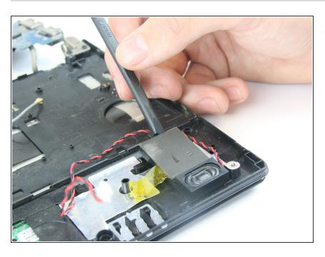
Using the spudger, lift the speaker up and out of it's holder, as shown.
