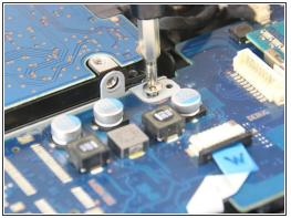
Use a Phillips #0 screwdriver to remove the six 4.5mm screws holding the motherboard to the case.
