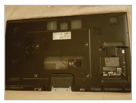
Remove the power cord and place the TV screen down on a soft surface, like a blanket.
