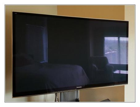
Remove the TV from the stand and place glass down on a flat, soft, and clean surface where you will have easy access to all four sides of it.
