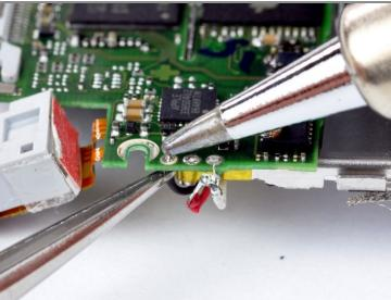
• De-solder the remaining leads, following the procedure illustrated in the previous step.
