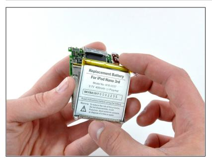
Place the new battery in the metal battery tray, sticking it down to the adhesive.
