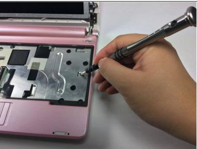
With the Phillips #1 screwdriver, remove the six screws that connect the metal plate to the motherboard.
