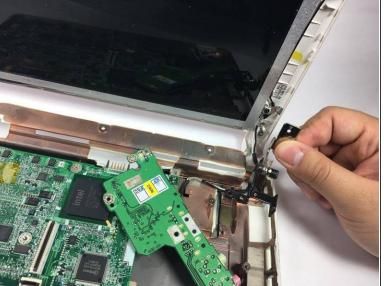
• Remove the hinge by holding on to the metal piece and pull towards yourself.
