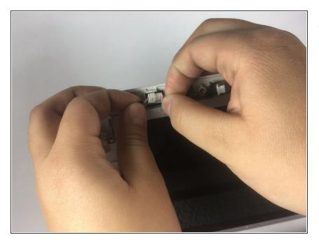
Disconnect the microphone, which located left of the camera piece, by pinching the tape around the wires, pinching the microphone, and pulling the two in opposite directions. This microphone is detached in the same way the camera was detached.
