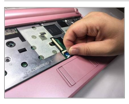
With your fingers, pull the blue plastic tab connected to the white connector at the bottom of the laptop to disconnect the trackpad from the motherboard.
