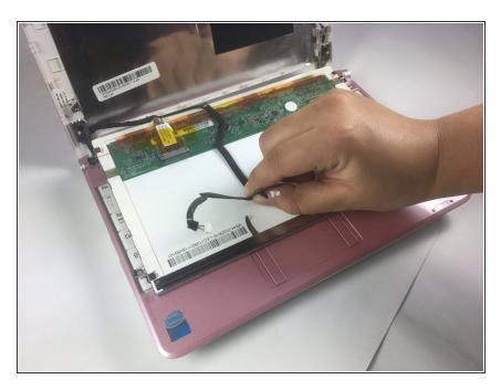
Gently peel off the black wire connected to both the microphone and the camera. This is attached with a small amount of adhesive to the back of the display screen.
