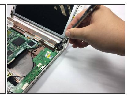
Remove the four screws located on the right green circuit board.
