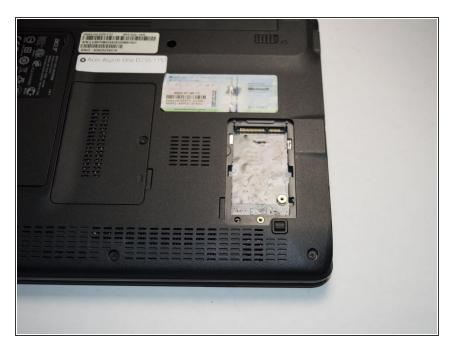
• Slide the 3G card forward until it is not connected.
