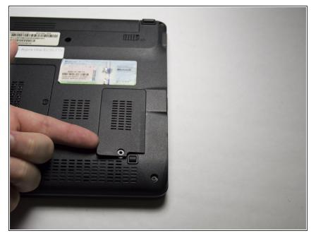
Open the panel by lifting up in the small groove using a finger, Plastic Opening Tool or similar device.
