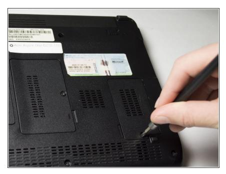
Unscrew the smallest panel using a Philips PH1 screwdriver in a counterclockwise motion.
