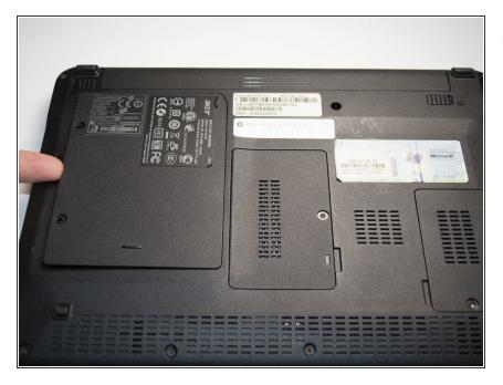
Lift the panel with your finger to reveal the hard drive.
