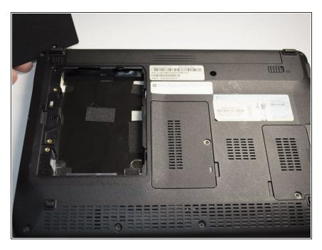
Slide the hard drive towards the battery until it is no longer connected.
