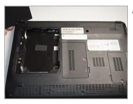
Lift the hard drive out of the compartment.
