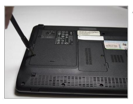
Unscrew the Largest panel using a Philips PH1 screwdriver in a counterclockwise motion.
